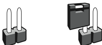
Feature " Off " (Jumper on one pin)
