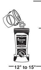
Leave 12" to 15" above and around Perform-Max to allow room for easy refilling.
