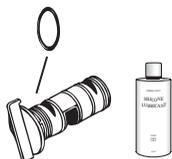
4. Carefully replace the rubber o'ring without stretching it. Squeeze a little silicone lubricant that came with your Perform-Max directly on the o'ring and spread it over o'ring surface with your finger.
