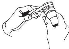
**1.** Apply teflon tape to the threaded end of both hose adapters.
