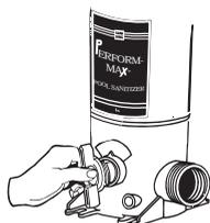
5. Carefully Insert control dial back into housing.
