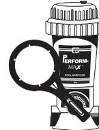
4. Use the handle end of cap tool if the dial is hard to turn.
