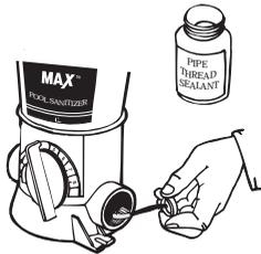
Following pipe thread sealant directions, brush sealant onto Perform-Max threads in both ports.
