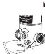
4. Unscrew drain knob in front of Models 910 and 930 and back of Models 940, 960, and 980. Allow all water to drain.
