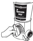
5. Push control dial completely into the housing and turn the dial to setting 2.
