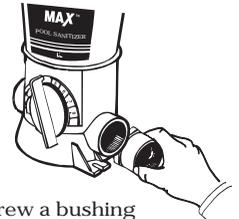
Screw a bushing into each port of Pool Sanitizer and hand tighten.
