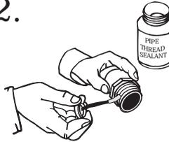
Brush sealant on the threads of both bushings.
