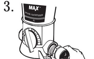
Screw a male adapter into each port of Perform-Max and hand tighten.
