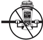
Do NOT install an inline Perform-Max off-line as this Perform-Max is different than an off-line unit.
