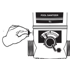
3. Unscrew side knob on Models 910 & 930 or cap knob on Models 940, 960 & 980 to relieve pressure.
