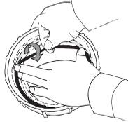
2. Take hold of the far end of the o'ring with the thumb and index finger of the other hand. Roll o'ring slightly back towards you
