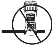
Do NOT install an off-line Perform-Max inline as this Perform-Max is different than an inline unit.
