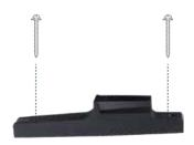
**EACH FOOT** Is mounted to the surface with two screws.
