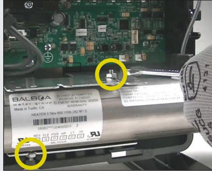
– Tighten the 2 nuts to secure the heater in place.
