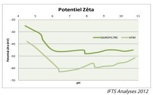
A controlled attack (patented process) of the glass matrix of AFM<sup>®</sup> grains exposes chromium oxide (green dye in glass) and silanol (SiO)- groups which, in the presence of oxygen, carry a strong negative charge. This causes an increase of 40% in zeta potential, from approximately -30 mv for untreated glass to -65mv for AFM<sup>®</sup>. The results of independent laboratory analyses are presented in the graph above.
