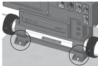
Now firmly attach unit to wooden base by using the remaining (2) screws backed by (2) washers to fix the front of the foot.
