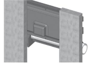
**Note:** Make sure these (2) screws and (2) washers are installed. They will make the pack stable when input, outputs and accessory connectors will be inserted in their ports.
