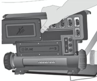
Release the 2" heater nuts from both ends of the spa piping. Release the in.xe™ Spa Pack by sliding the unit away from the guide plate that holds the backside of the unit's feet in place.
