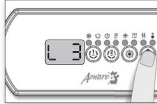
Use the **Up/Down** key to choose the new desired low level configuration number.
