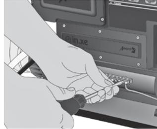
Disconnect the grounding cable from the Bonding Lug of the in.xe™ Spa Pack.
