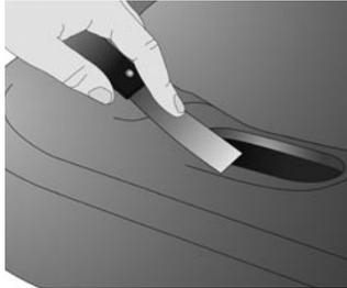
With an scraper tool, gently clean the surface of installation of the new keypad, finish the job with an alcohol saturated paper towel to remove any unwanted residue left over from the old keypad.
