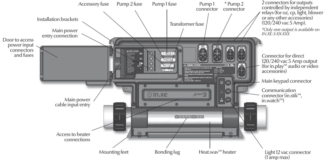
**Note: No connectors should remain unplugged. Use blank plugs to fill unused connectors.**
