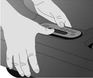
Secure the keypad in place. Insure that its adhesive strip is properly glued by pressing evenly with your finger over the entire surface.
