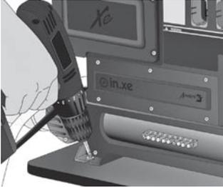
Remove the 2 screws that hold the front of the unit's feet attached to the spa floor.
