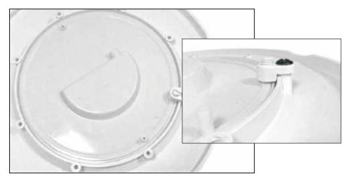
Spectravision replacement lamps are supplied complete with adjustable plastic lamp clamps which are fixed to light face ring using the original lamp housing screws.
