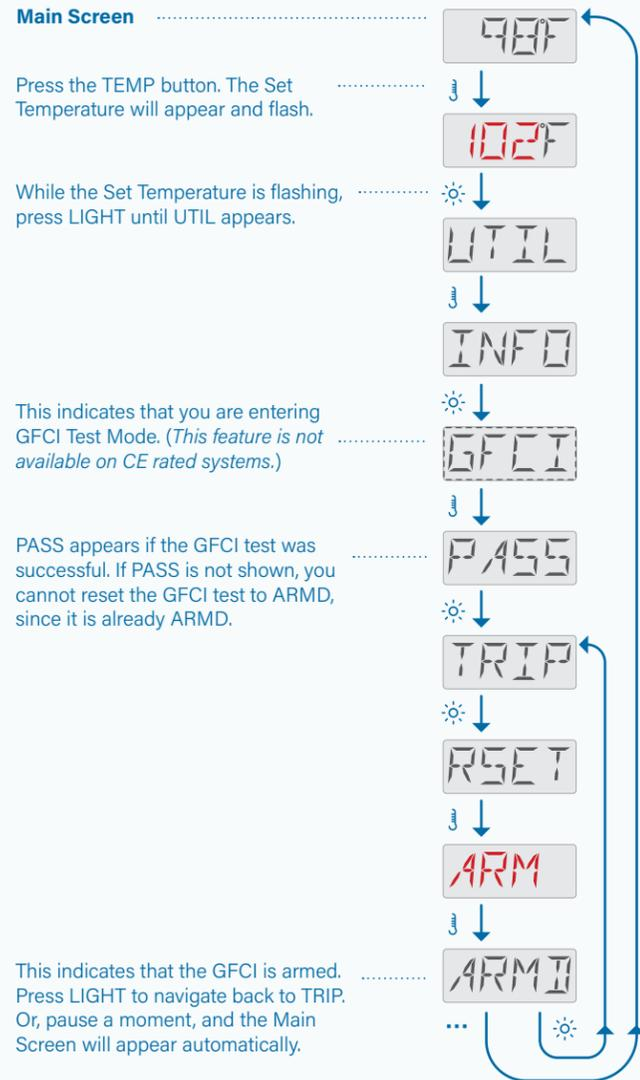
Follow this sequence to check the current status of the GFCI test feature.
