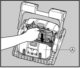
2. Insert the internal suction adaptor into the robot. It should be placed in the side of the robot that has the pipe connection door hatch on it (A). Press the adaptor against the right wall and lower it (see the direction arrow on the adaptor) until it reaches the suction inlet.
