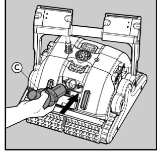
5. Connect the suction pipe to the swivel connector by pressing the pipe against the black locknut. Do not tighten the pipe against the locknut. Ensure that there is a small space between the locknut and the pipe (D).
