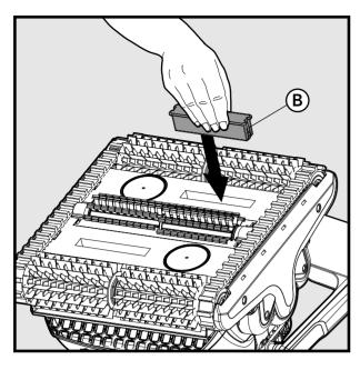
3. Insert the suction inlet plug into the suction inlet which is on the opposite side from where the suction adaptor is installed. To remove the suction inlet plug, press the tabs (B) on both sides of the plug and pull.
