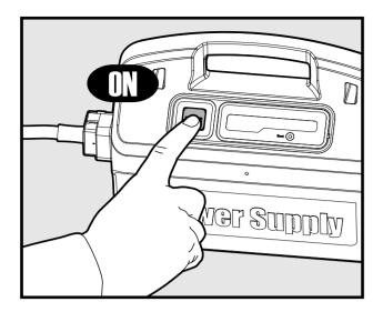
Switch the power supply on. The robot will now begin working for a complete cleaning cycle. At the end of the cycle, it will automatically switch itself off.
