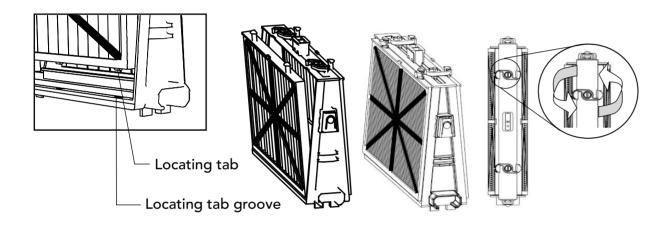
Reinstall the base frames with filters according to the diagram.
