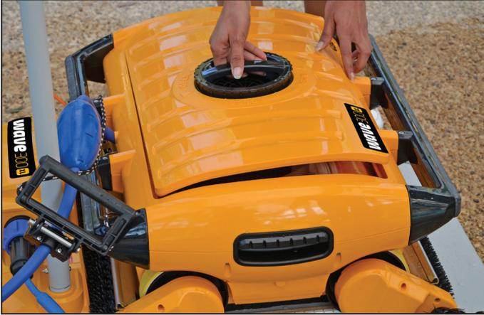
2. Remove the 2 filter bags from the robot.
