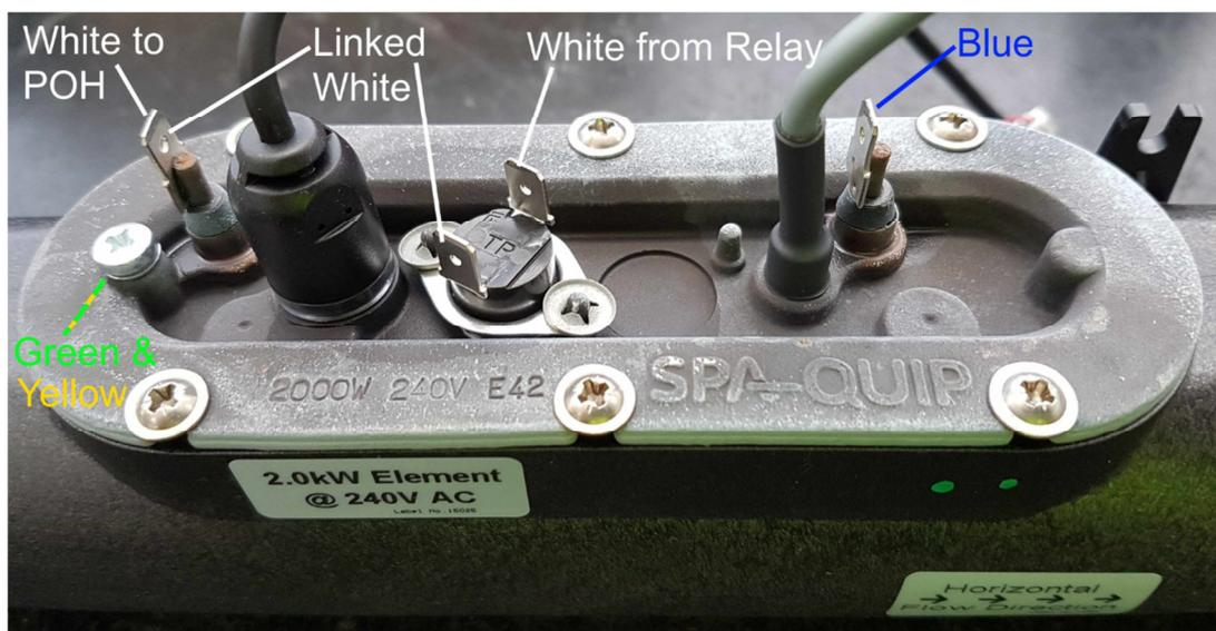
Incoloy Heater Element pre Nov 2015 wiring connections
