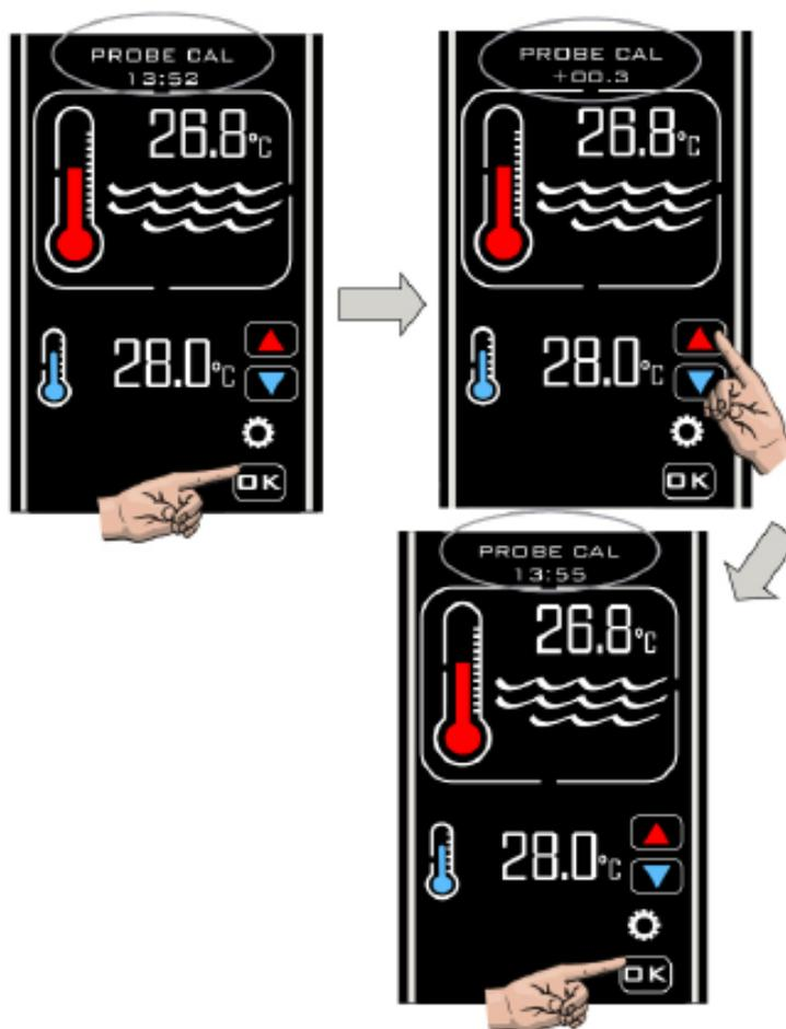
Probe calibration is usually not required. However, should you need to make an adjustment take a temperature reading from the pool water with an accurate thermometer then adjust as required.
