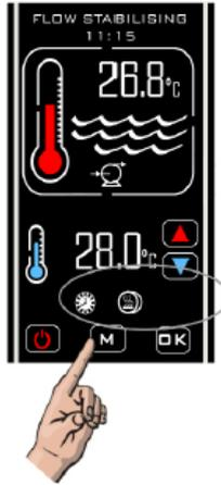
In this mode the controller will heat whenever it is receiving flow during a timed-on period.
