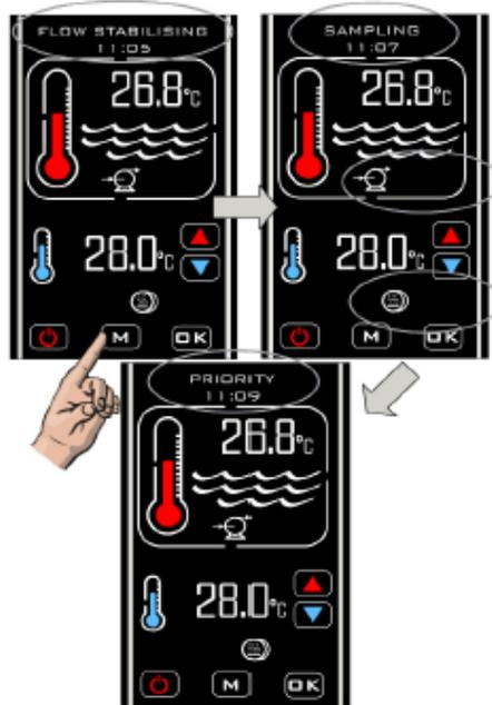
Once the **'Priority of Heating'** feature has been enabled the controller will take a water temperature sample every hour and the message **'SAMPLING'** will be displayed.
