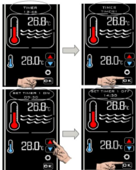
The timer mode allows you to set up 4 on and off time periods when you would like heating to take place. These can be set to take advantage of off-peak energy tariffs, or to ensure your pool is at the required temperature during specific time periods.
