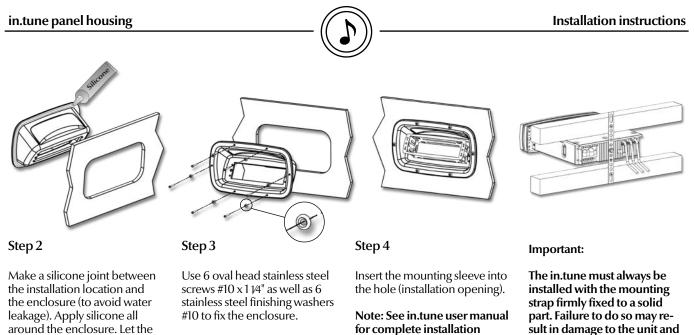
around the enclosure. Let the silicone dry and remove excess.
