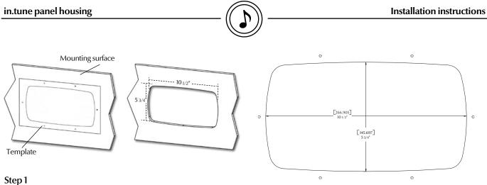
Using the drilling template supplied with the unit, determine the mounting location and then stick the template on the location.
