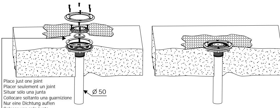
Prefabricated Pool with Liner Assembly / Montaje Piscina Prefabricada con Liner
