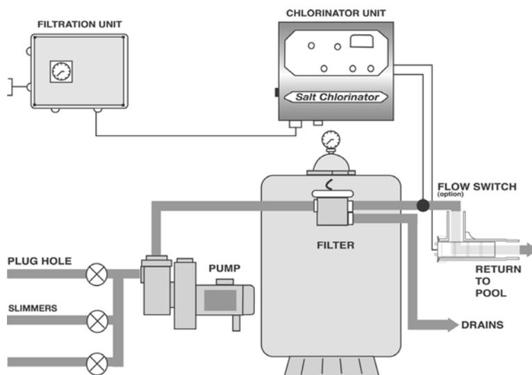
The chamber must be attached to the return pipe (50 or 63) that runs towards the swimming pool, after the filter and after the heater or the start of the compressor. Ensure that there is sufficient room on the removable side of the chamber so that one can remove the electrode.
