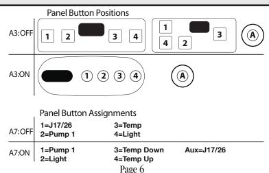
**Blower or 1-speed Pump 2 is required**, connect to J17/26. For no Blower and no Pump 2, use GS500Z or GS515Z.
