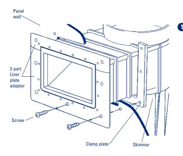
Pass skimmer throat through panel wall aperture (see previous page for details) and clip 2-part liner plate adaptor onto recess on skimmer throat. Push skimmer back through wall until liner adaptor touches panel wall and all seven holes are aligned.
