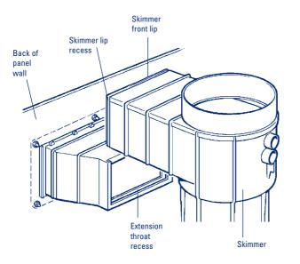
Using a brush, apply ABS cement to the front lip and recess of the Certikin skimmer and to the recess in the back face of the extension throat. Slot the skimmer lip down into the slot in the throat until firm. (The two holes in the base of the throat recess allow excess cement to squeeze out, ensuring an all-round fit). Using the brush, smooth off any other excess cement and re-coat the joins of the skimmer-throat inside and out, filling any voids to ensure a watertight seal.
