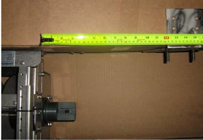
3. Place the fixed mounting plate to the back of the pit. Secure the fixed mounting plate to the back of the pit wall by using the four pre drilled holes and fasten.
