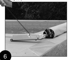
Hold down the button on the remote control and walk with the WALU COOL until your cover is fully rolled up.
