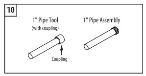
10. Create a 1" pipe tool with coupling attached to install the pipe assembly in the following steps.
