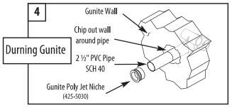
4. While guniting, scoop out gunite around the  $2\,\%$ " PVC pipe, allowing room for the plaster niche (425-5030).
