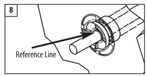
8. Draw a reference line on the 1" PVC pipe, flush with the back edge of the measuring tool.
