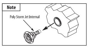
Note: To winterize the jet system, remove the jet internal from the wall fitting ONLY. Install a #10 rubber expansion plug inside of the fitting opening.
