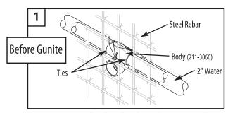
1. Hang Poly Storm Gunite Jet Body with ties through preset holes onto steel rebar.
