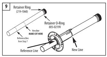
9. Remove the 1" pipe assembly from the jet body assembly and realign the measuring tool with the reference line. Make a new line at the Poly Storm Gunite Jet setback on the measuring tool.
