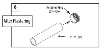
6. Cut a piece of 1" PVC pipe few inches longer than the 2  $\frac{1}{2}$ " pipe and glue the threaded retainer ring to one end.
