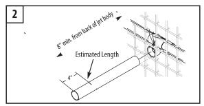
2. Estimate needed length of 2  $\frac{1}{2}$ " PVC pipe by thickness of wall. Cut 2  $\frac{1}{2}$ " PVC pipe at least 4" longer than estimated finish length. Then glue 2  $\frac{1}{2}$ " PVC pipe to body.
