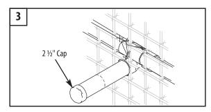
3. Glue 2  $\frac{1}{2}$ " cap onto end of pipe for pressure test before guniting.
