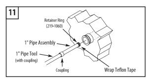
11. Install 4-6 wraps of Teflon tape around the threaded Retainer Ring, including 1 wrap over the o-ring. Dry fit the pipe tool with coupling on the end of the 1" pipe assembly. Thread the assembly into the body assembly until it is snug and the pipe tool with coupling spins freely. Remove the pipe tool from the end of the pipe assembly.
