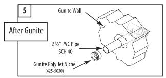
5. Before plastering, cut the  $2\,\%''$  pipe so that the plastic niche will fit flush with the finished wall. Glue the plaster niche onto the pipe, then cover the niche with tape for plastering.
