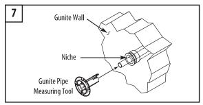
7. Insert 1" PVC pipe assembly through the niche and up to the jet body assembly and thread in. Slide the Gunite Pipe Measuring Tool (218–1960A) over the end of the pipe until flush against the plaster niche.
